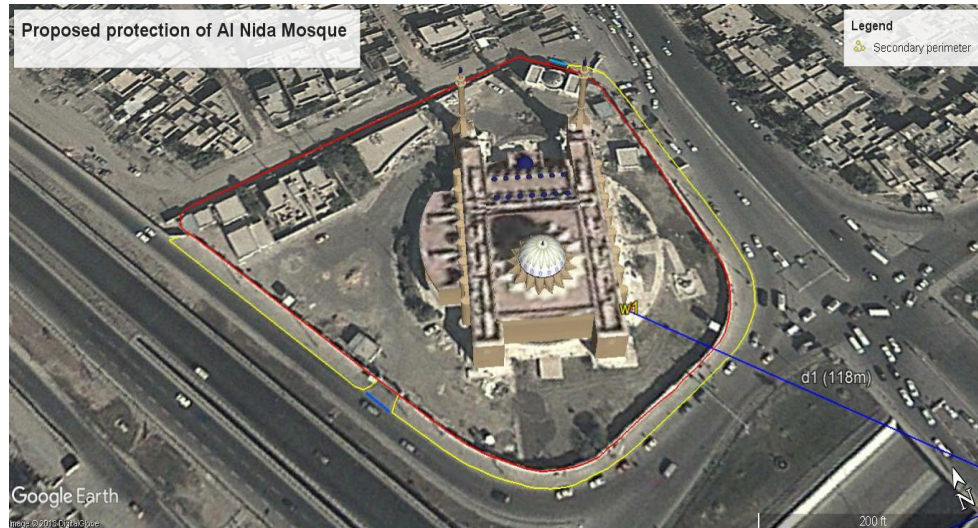
Fig. 7: Proposed barriers around the building [21]
